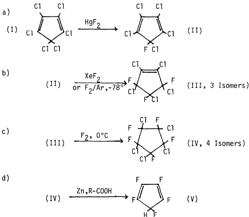
1,2,3,4,5 Pentafluorocyclopentadiene (V) is a very reactive diene. If pure, dimerisation occurs already at  $-78^\circ\text{C}$ , and is partially reversible at  $700^\circ\text{C}$ .
